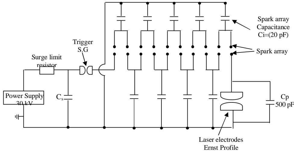
Fig. (2): Charge-transfer circuit used in this system.
