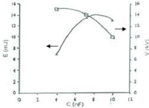
**Fig. (7):** Output laser energy and supply voltage vs. bank capacitance.
