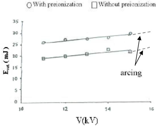
Fig. (3): Output laser energy vs supply voltage with and without preionizer.
